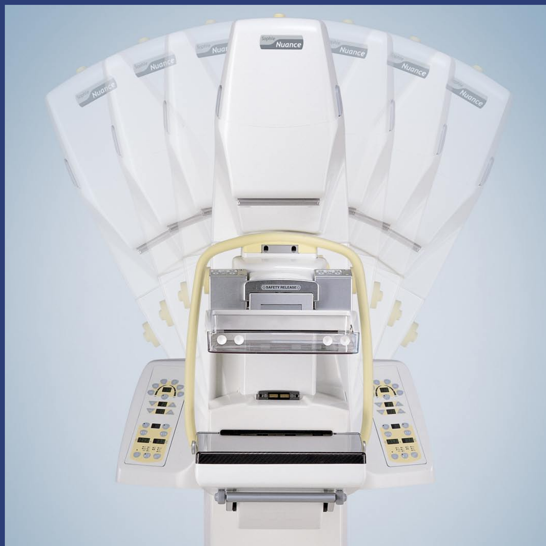
The prototype of the Planmed Nuance tomosynthesis full field digital mammography system
