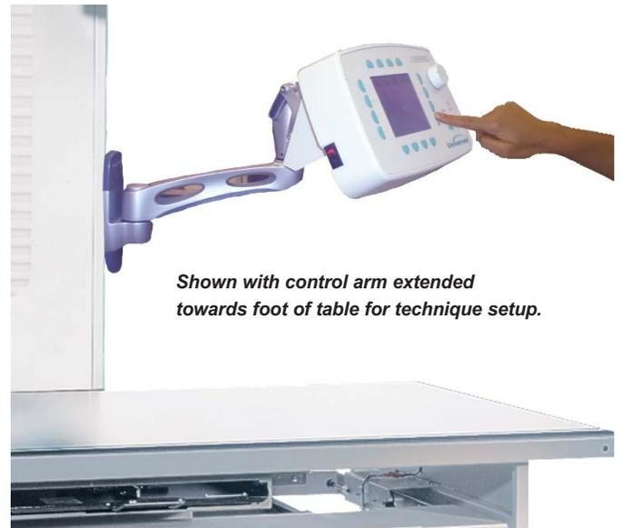
*Shown with control arm extended towards foot of table for technique setup.*
